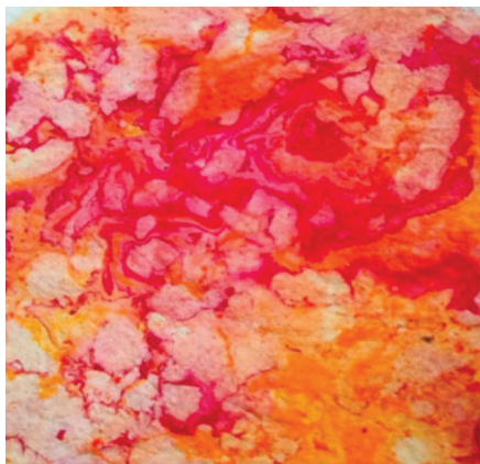
Fig. 5: Marbling effect with gum indulka and reactive dye
