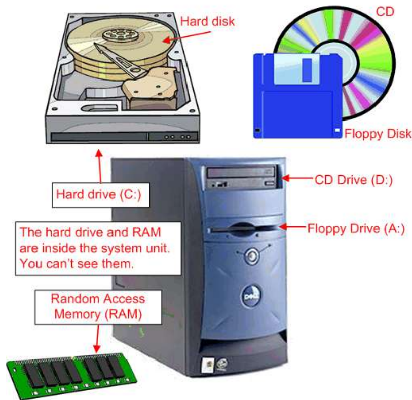
Figure 5.10: View of RAM,Hard drive,Floppy disk
